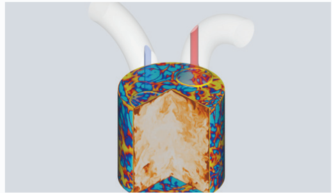
Instantaneous temperature distribution inside the cylinder and heat flux along the cylinder walls during the compression stroke in the TCC-III engine. Image: George Giannakopoulos, ETH Zurich
